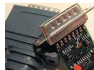
**Figure 7. Overmold PCBA solution.**
