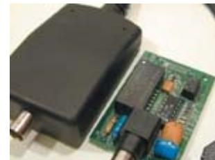
Figure 2. PCMCIA overmolded device.
