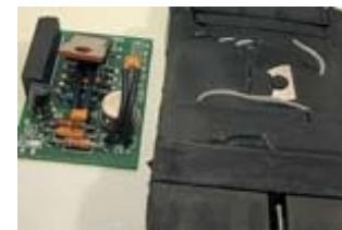
Figure 4. Direct premold, prior to overmold.
